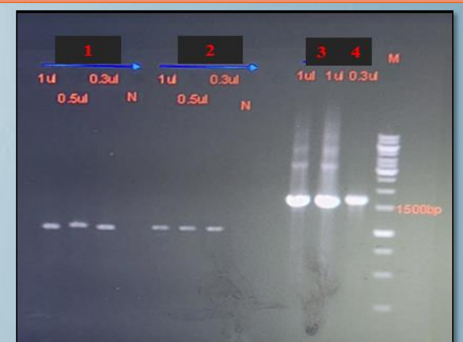
Figure 5. PCR activity results of Taq Polymerase produced and purified in our laboratory. Beta-Actin (1 and 2) and alpha-glucosidase (3 and 4) genes were amplified. 2 and 4) PCR result with commercial Taq polymerase (using genomic DNA). 1 and 3) PCR result (genomic DNA was used) performed with Taq polymerase produced in the laboratory.
